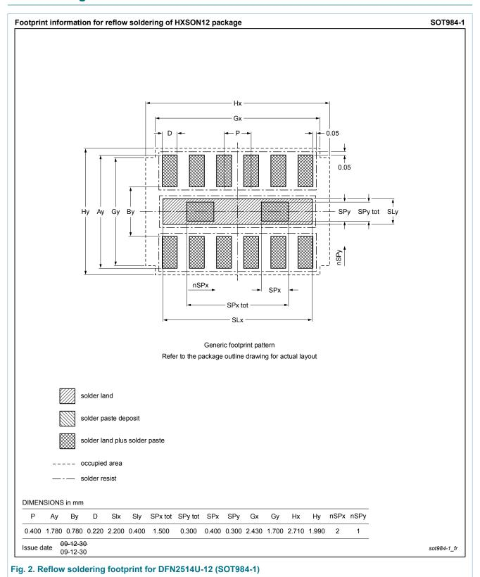
DFN2514U-12: plastic thermal enhanced extremely thin small outline package; no leads; 12 terminals
