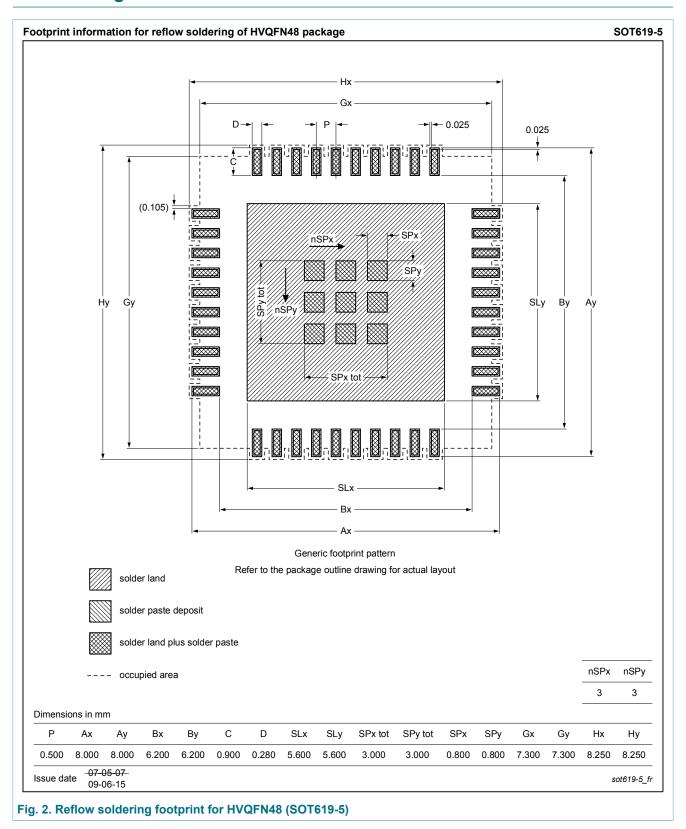
plastic thermal enhanced very thin quad flat package; no leads; 48 terminals; body 7 x 7 x 0.9
