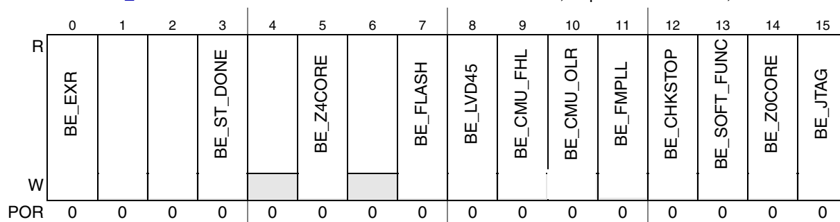
Figure 99. Functional Bidirectional Reset Enable Register (RGM_FBRE)
