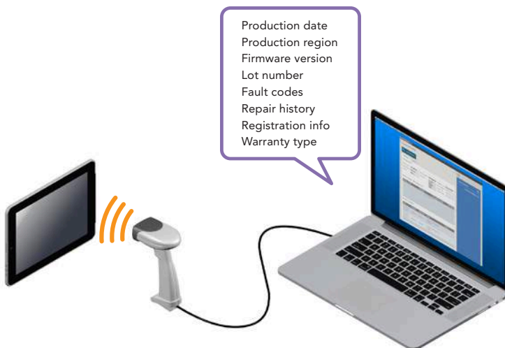
Figure 8 RFID tags embedded into products can store information that facilitates return logistics. Data can also be retrieved from inoperable devices.
