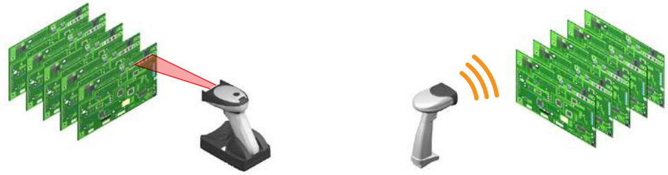
Figure 2 Unlike barcodes, RFID does not require line of sight to operate
