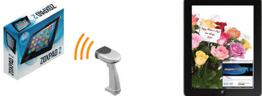
Figure 10 Using embedded RFID bridge ICs, retailers can access products within sealed packages to add additional features such as personalized messages or gift cards
