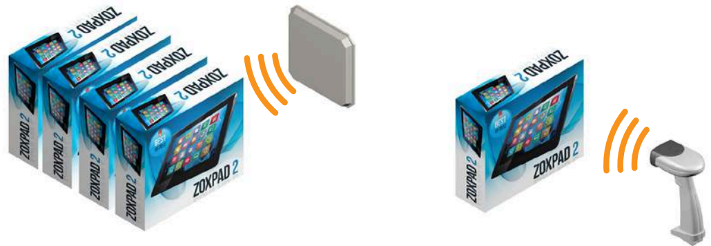
Figure 9 With embedded RFID bridge circuits, products can be deactivated after production, then activated at the point of sale to deter fraud and theft.
