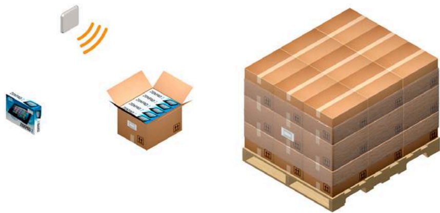
Figure 7 By replacing standard labels with RFID-encoded labels, readers can track individual items, cased products, and palletized products.
