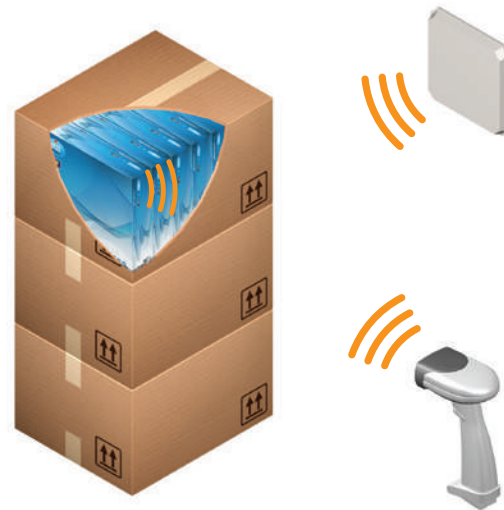
Figure 6 RFID tags are readable through most packaging
