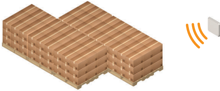
Figure 5 RFID readers can access item level identifying information of stored inventory
