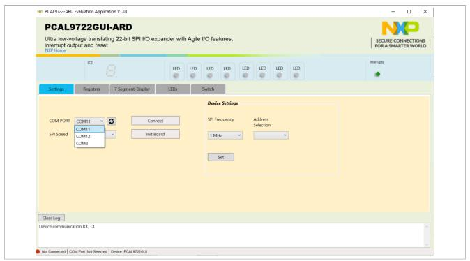
3. Use Setting tab to select SPI speed, and click on the "Init Board" button.
