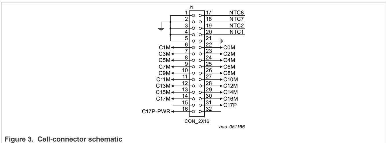
Figure 3. Cell-connector schematic
