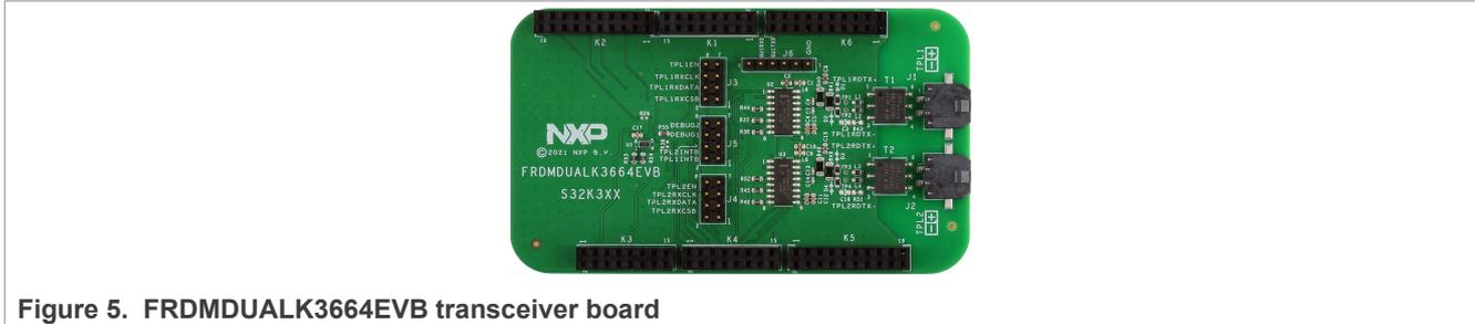
Figure 5. FRDMDUALK3664EVB transceiver board
