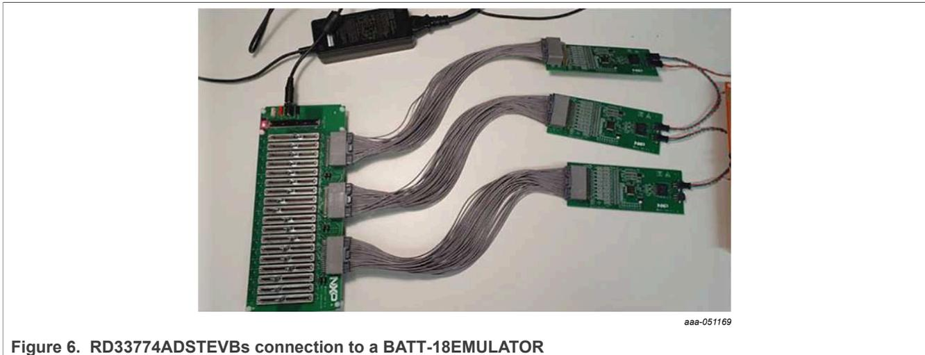
Figure 6. RD33774ADSTEVBs connection to a BATT-18EMULATOR
