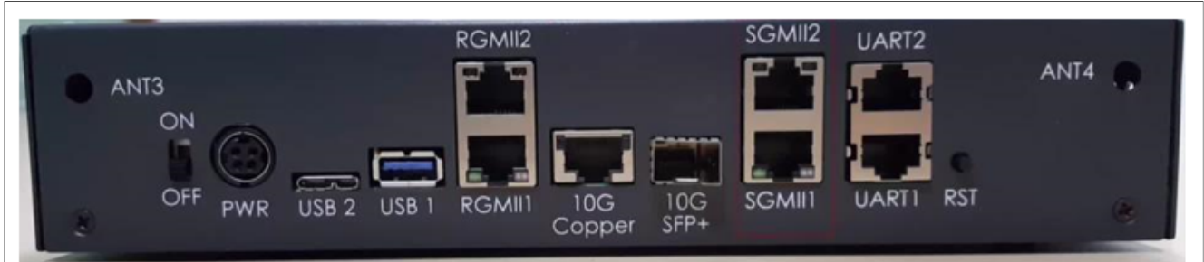
Figure 187. LS1046ARDB port layout
