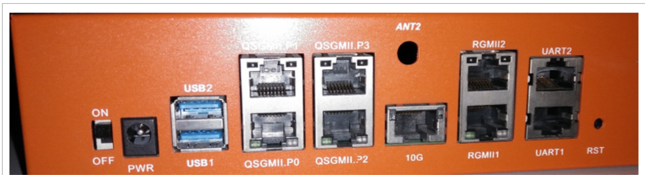
Figure 185. LS1043A Port Layout
