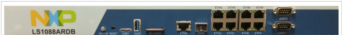
Figure 190. LS1088ARDB Port Layout
