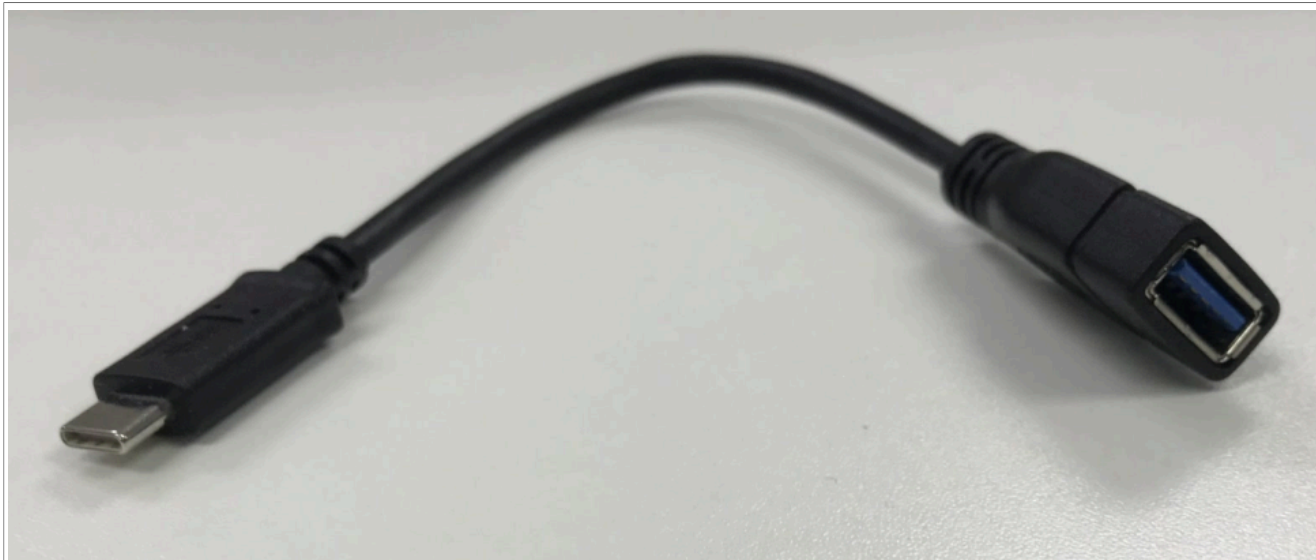
Figure 32. USB 3.0 Type-C cable
