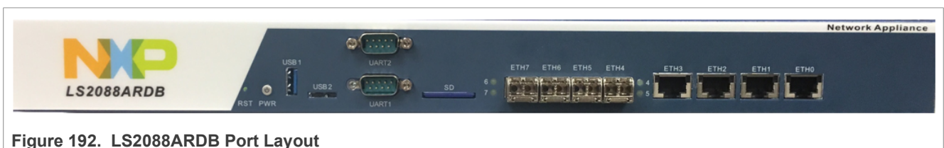
Figure 192. LS2088ARDB Port Layout
