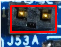
Figure 17. Open jumper J53 to configure the device as LIN slave
