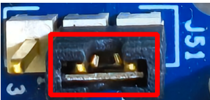
Figure 18. Short pins 1 and 2 of J51 to allow transfer of CP data through LIN slave
