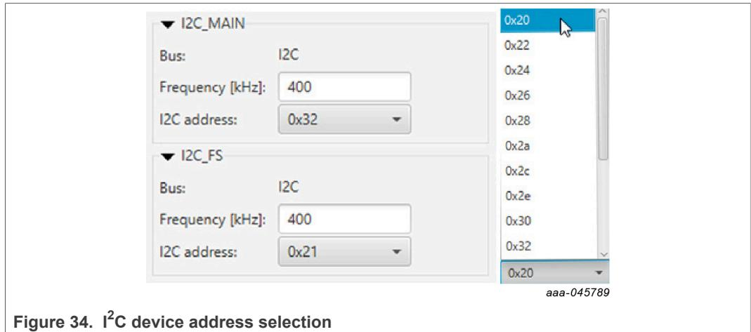
Figure 34. I<sup>2</sup>C device address selection
