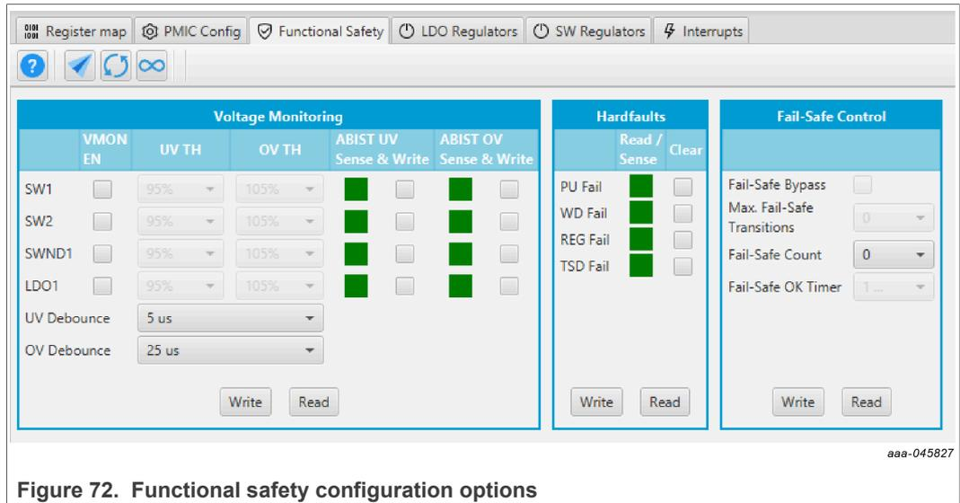
Figure 72. Functional safety configuration options
