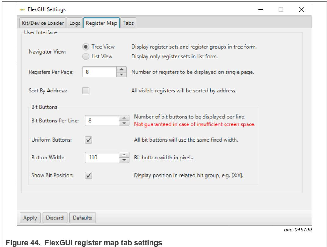
Figure 44. FlexGUI register map tab settings
