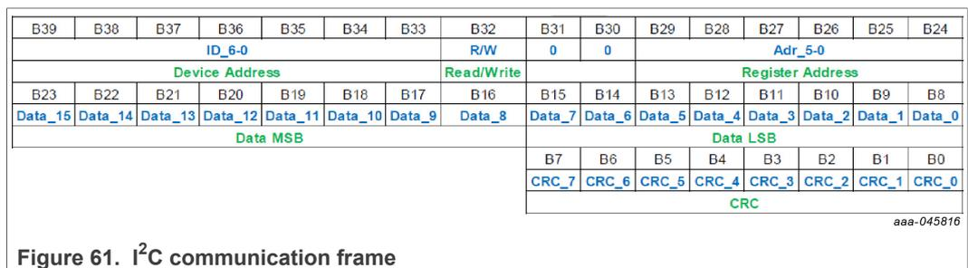
Figure 61. I<sup>2</sup>C communication frame
