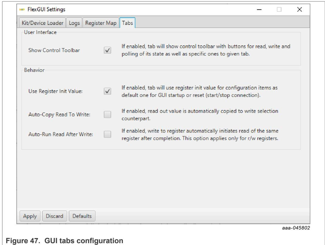
Figure 47. GUI tabs configuration
