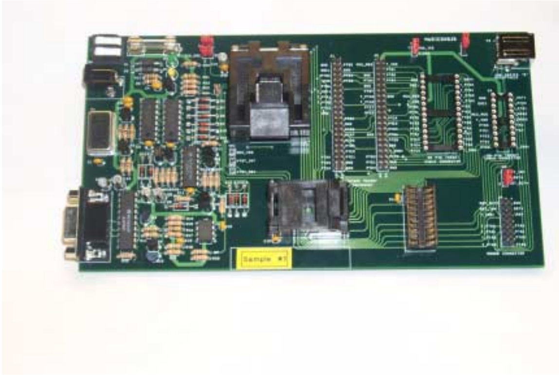
Figure 1-1 M68ICS08JB In-Circuit Simulator Board
