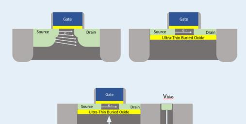
**Body Biasing**: Faster when required and more energy efficient when performance isn't as critical
