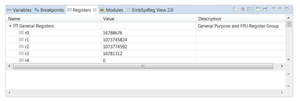
View peripheral registers in the EmbSysReg tab
