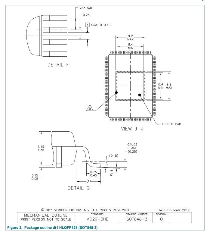
HLQFP128, plastic, thermal enhanced low profile quad flat package; 128 terminals; 0.5 mm pitch; 14 mm x 20 mm x 1.4 mm body
