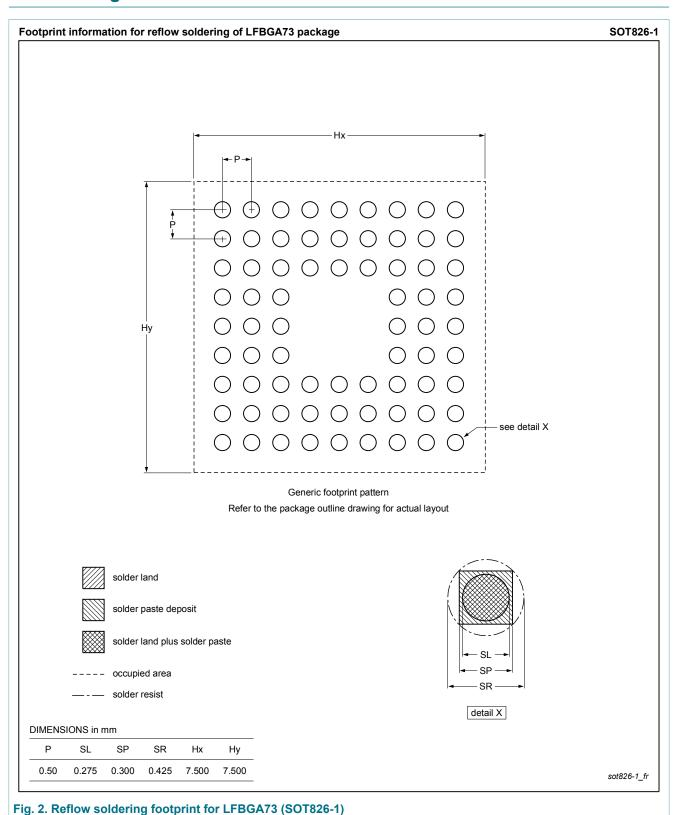
plastic low profile fine-pitch ball grid array package; 73 balls; body 7 x 7 x 0.9 mm
