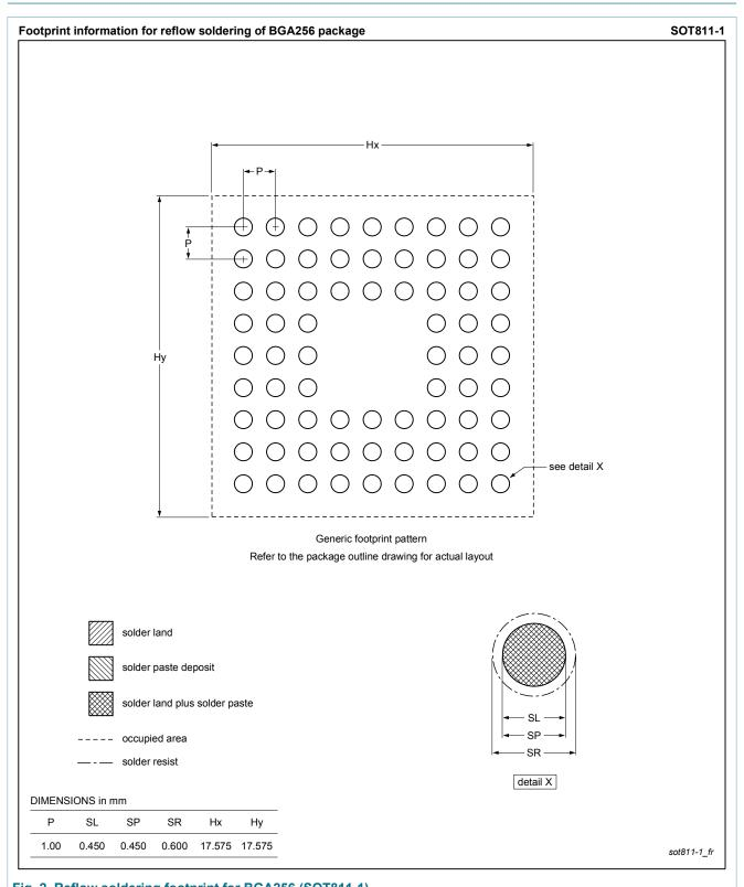
plastic ball grid array package; 256 balls; body 17 x 17 x 1.2 mm
