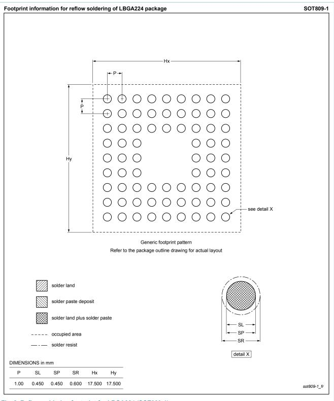
Fig. 2. Reflow soldering footprint for LBGA224 (SOT809-1)
