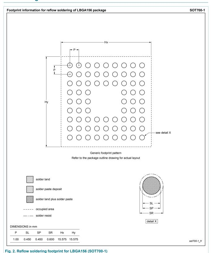
plastic low profile ball grid array package; 156 balls; body 15 x 15 x 1.05 mm
