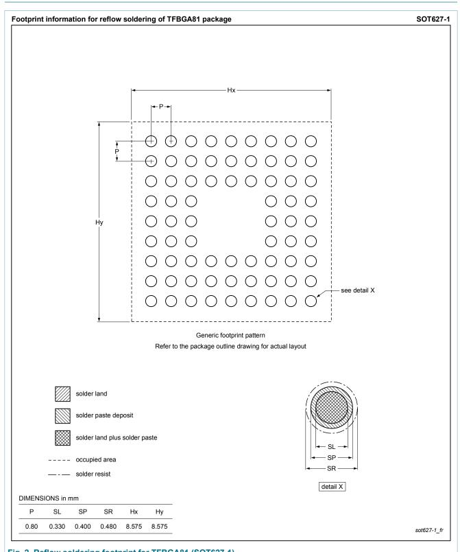
Fig. 2. Reflow soldering footprint for TFBGA81 (SOT627-1)
