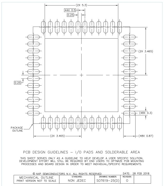
Fig. 5. Reflow soldering footprint part2 for HVQFN48 (SOT619-25(D))
