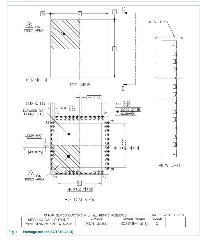
plastic thermal enhanced very thin quad flat package; no leads; 0.1 dimple wettable flank, 48 terminals; 7 mm x 7 mm x 0.9 mm body
