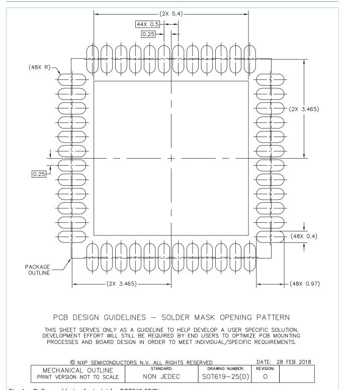
Fig. 4. Reflow soldering footprint for SOT619-25(D)
