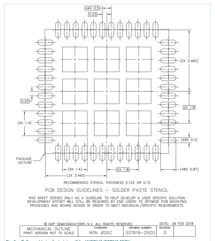
Fig. 6. Reflow soldering footprint part3 for HVQFN48 (SOT619-25(D))
