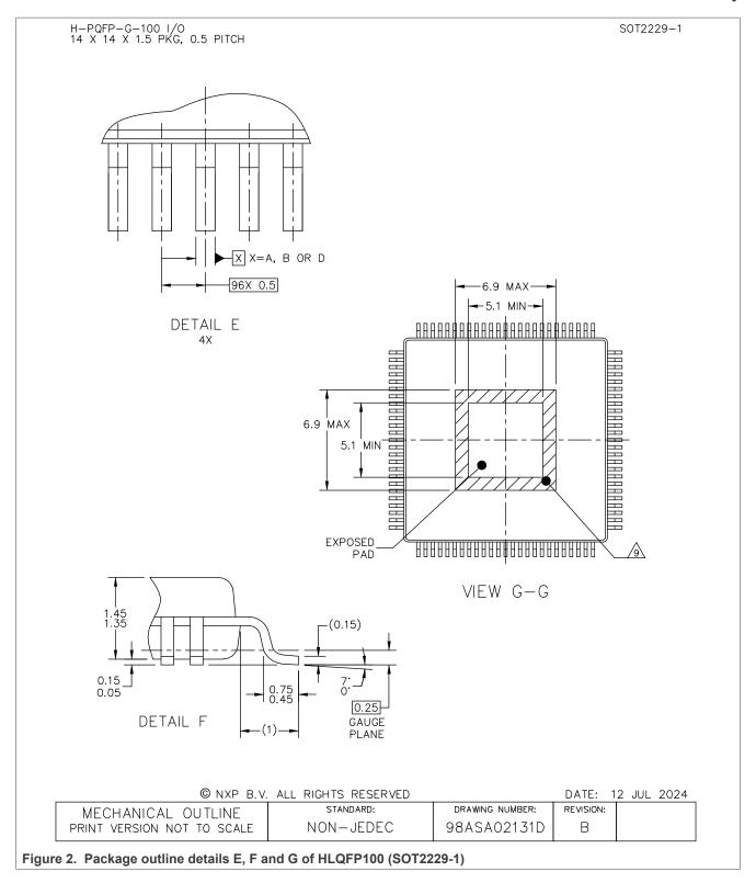
HLQFP100, plastic, thermal enhanced low profile quad flat package; 100 terminals; 0.5 mm pitch; 14 mm x 14 mm x 1.5 mm body
