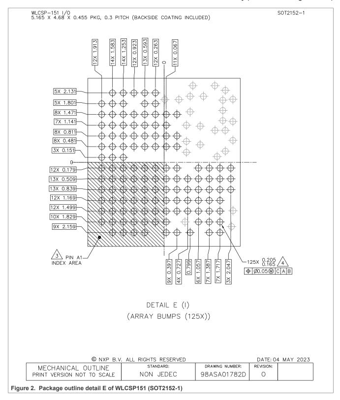
WLCSP151 wafer level chip-size package, 151 terminals, 0.3 mm pitch, 5.165 mm x 4.68 mm x 0.455 mm body (backside coating included)
