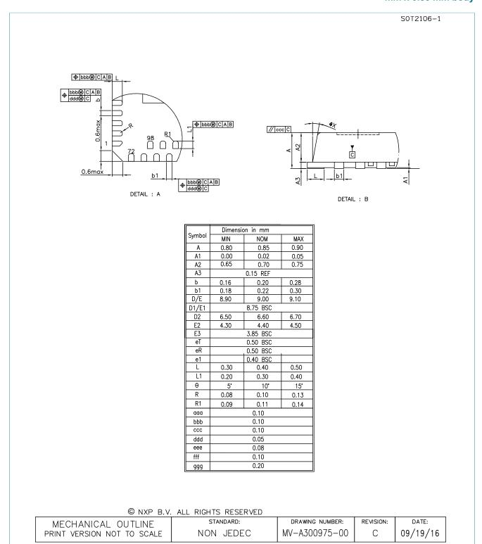
Figure 2. Package outline detail HVQFN98 (SOT2106-1)
