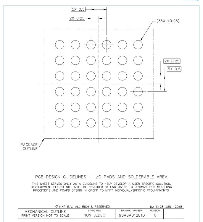
Figure 4. Reflow soldering footprint part2 for VFBGA36 (SOT1985-1)
