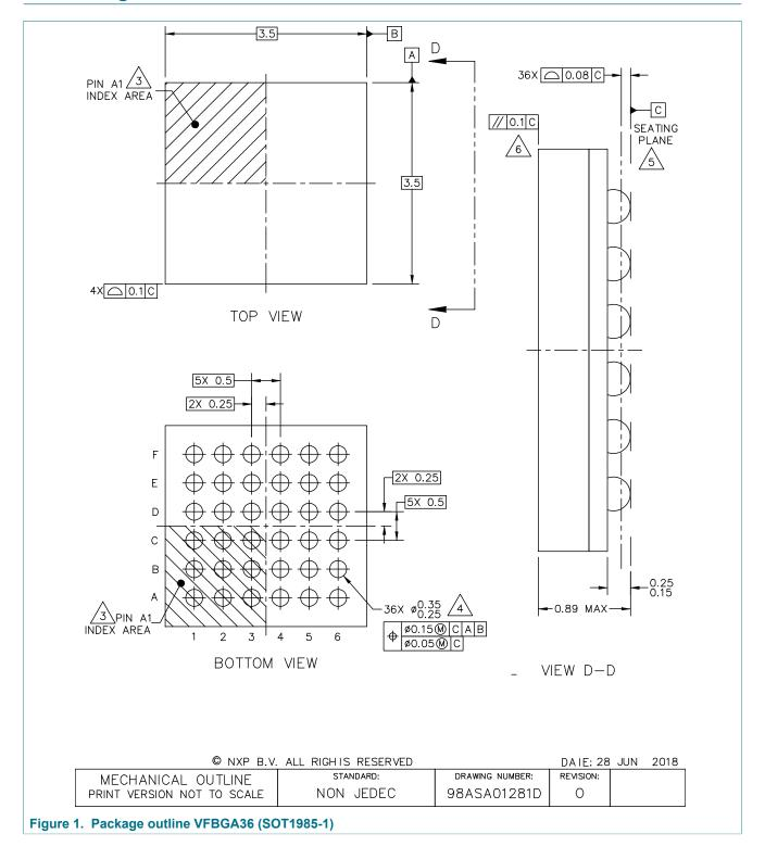
VFBGA36, very thin fine-pitch ball grid array package, 36 terminals, 0.5 mm pitch, 3.5 mm x 3.5 mm x 0.8 mm body
