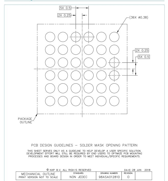
Figure 3. Reflow soldering footprint part1 for VFBGA36 (SOT1985-1)
