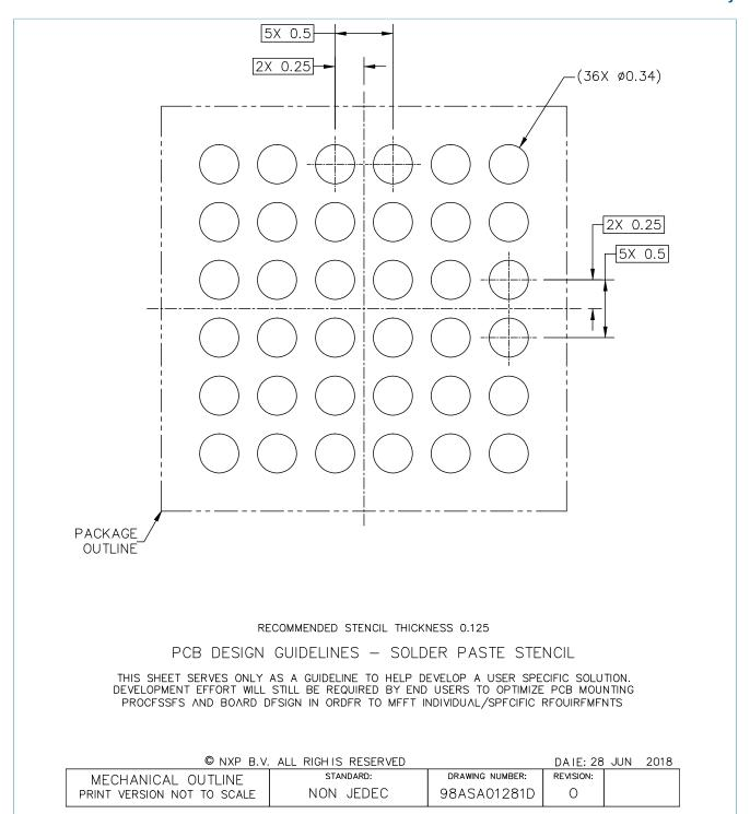
Figure 5. Reflow soldering footprint part3 for VFBGA36 (SOT1985-1)
