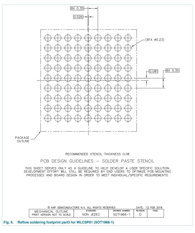
WLCSP81, wafer level chip-scale package; 81 bumps; 0.35 mm pitch, 3.55 mm x 3.36 mm x 0.365 mm body
