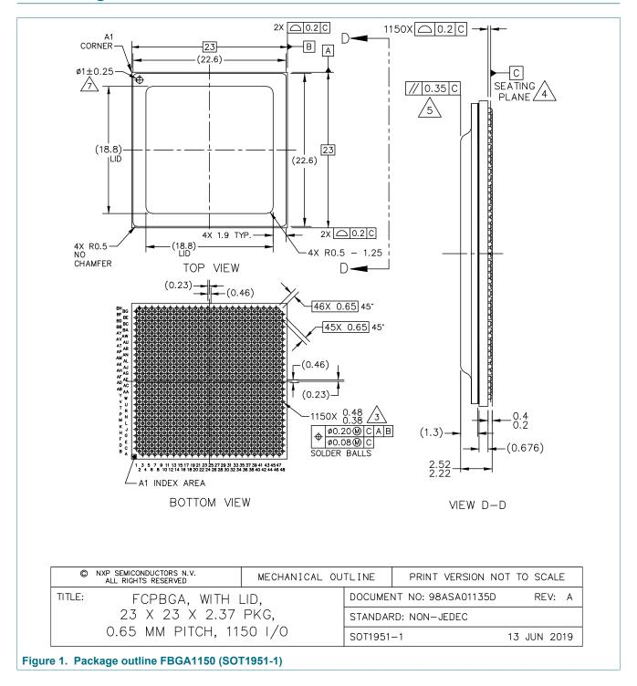
FBGA1150, plastic, fine-pitch ball grid array package, 1150 balls, 0.65 mm pitch, 23 mm x 23 mm x 2.37 mm body
