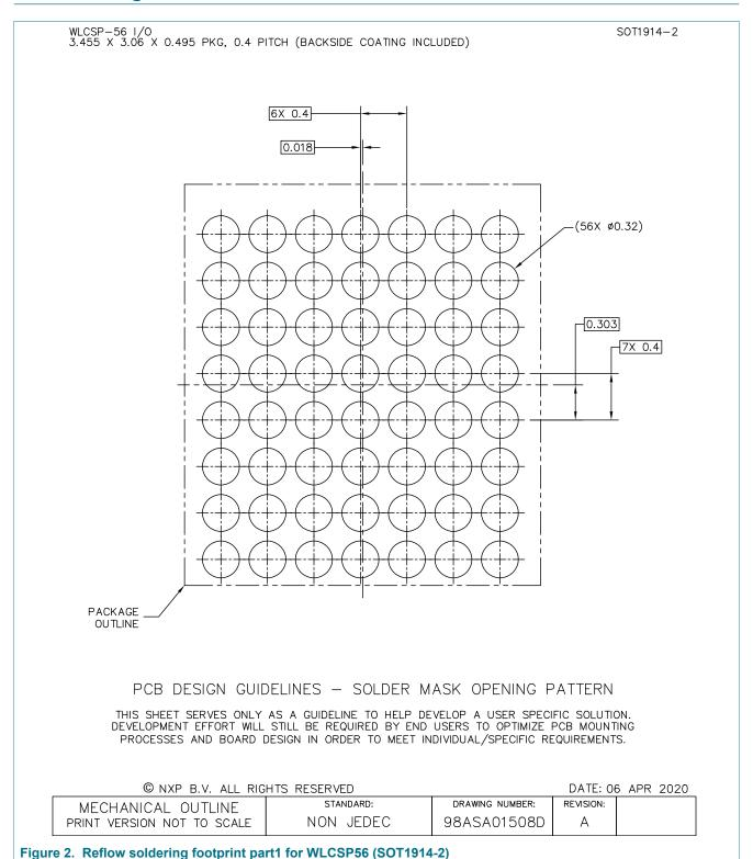
WLCSP56, wafer level chip-scale package; 56 bumps, 0.4 mm pitch, 3.455 mm x 3.06 mm x 0.495 mm body (backside coating included)
