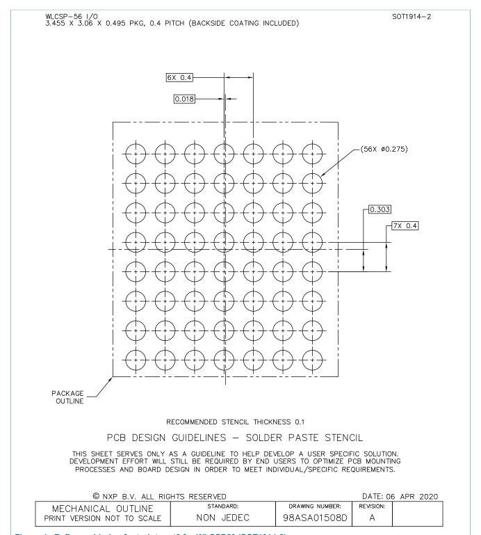
Figure 4. Reflow soldering footprint part3 for WLCSP56 (SOT1914-2)
