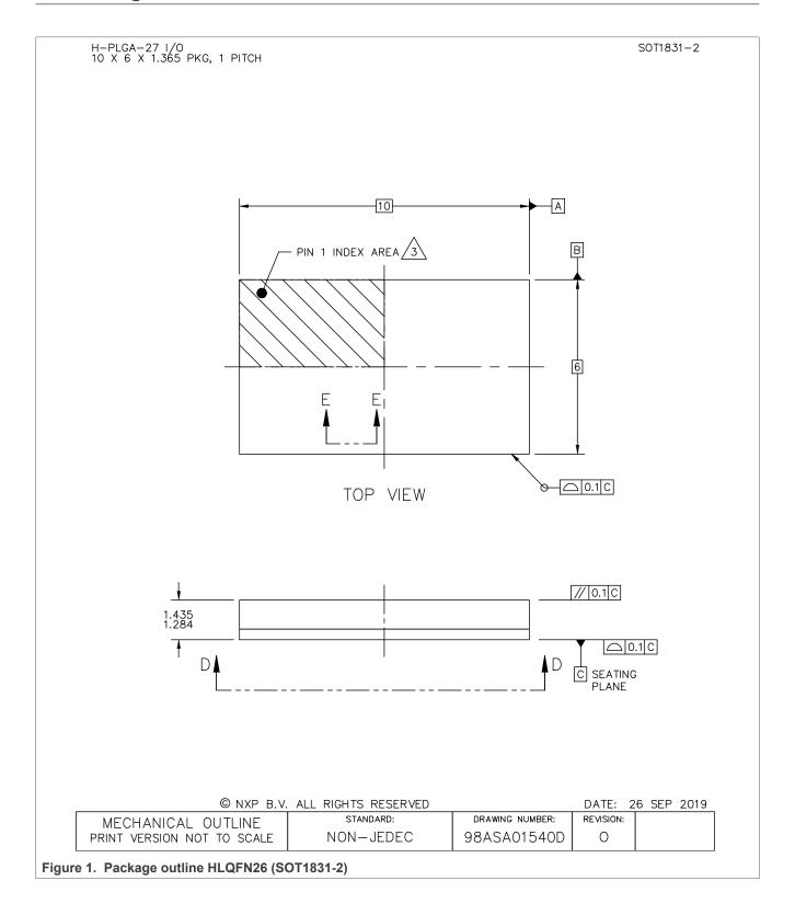
HLQFN26, thermal enhanced low profile quad flat package, no leads, 1 mm pitch, 10 mm x 6 mm x 1.365 mm body
