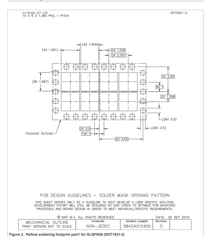
HLQFN26, thermal enhanced low profile quad flat package, no leads, 1 mm pitch, 10 mm x 6 mm x 1.365 mm body
