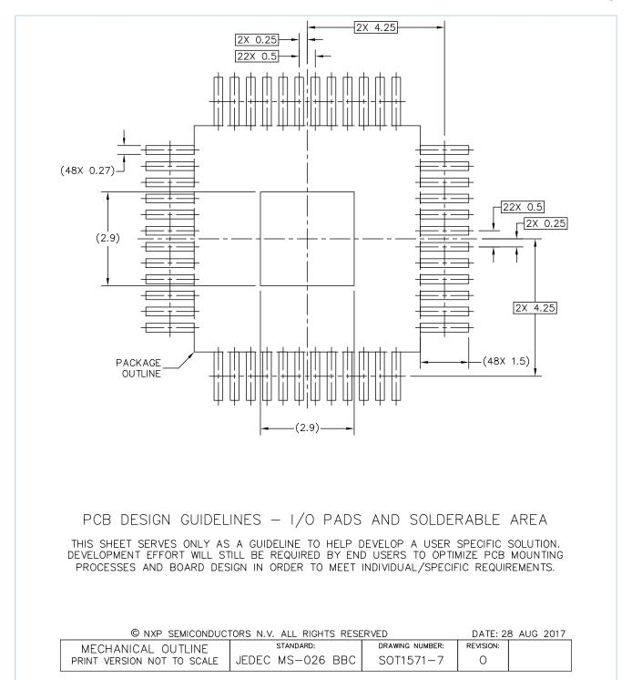
Fig. 5. Reflow soldering footprint part2 for HLQFP48 (SOT1571-7)
