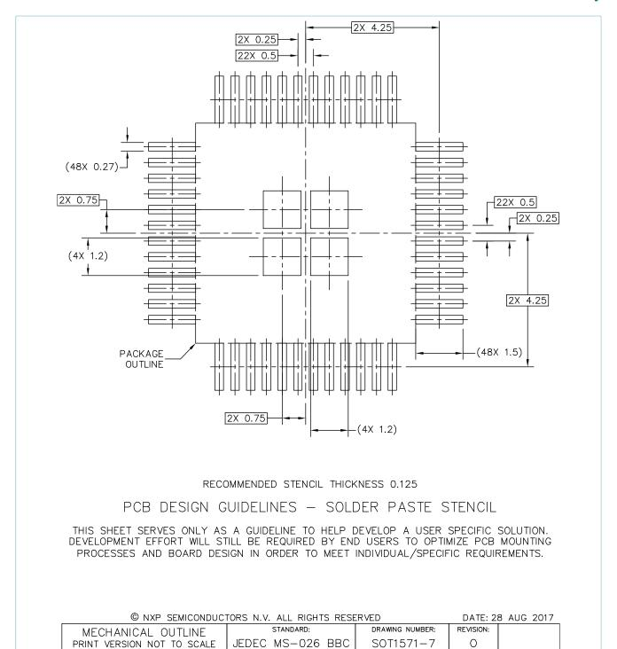
Fig. 6. Reflow soldering footprint part3 for HLQFP48 (SOT1571-7)
