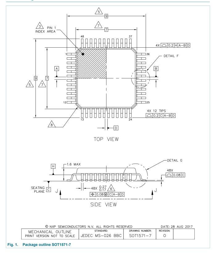
plastic, thermal enhanced low profile quad flat package; 48 leads; 0.5 mm pitch, 7 mm x 7 mm x 1.4 mm body
