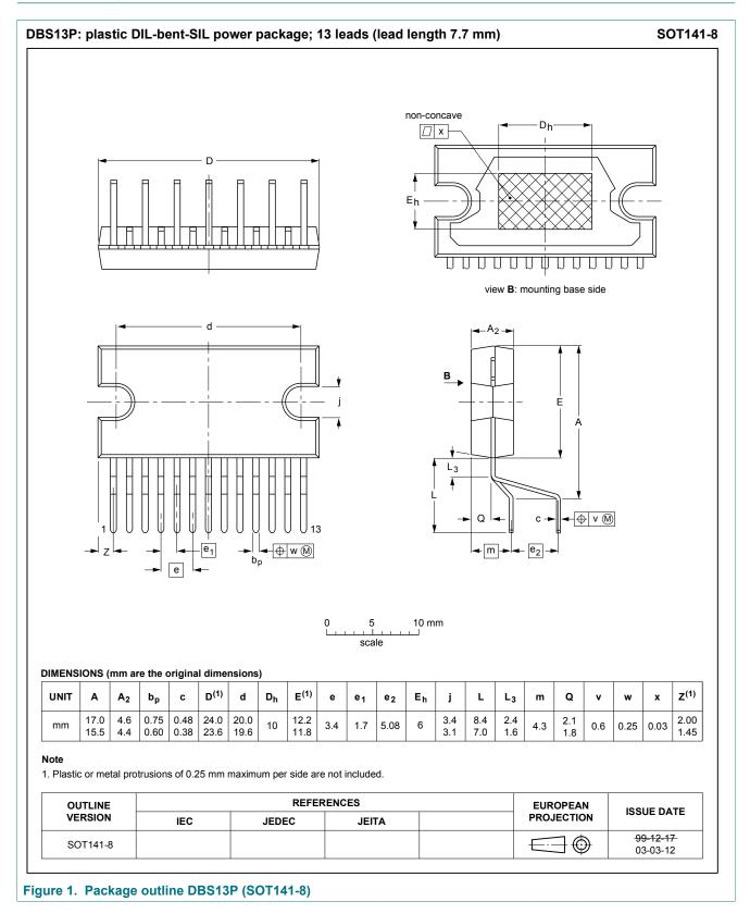
plastic DIL-bent-SIL power package; 13 leads (lead length 7.7 mm)
