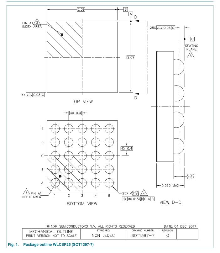
WLCSP25, wafer level chip-scale package; 25 bumps; 0.4 mm pitch, 2.09 mm x 2.09 mm x 0.525 mm body
