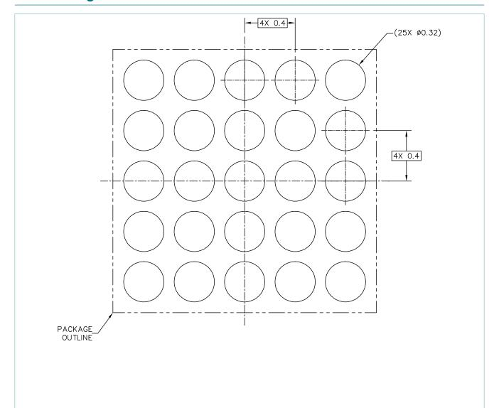
PCB DESIGN GUIDELINES - SOLDER MASK OPENING PATTERN
