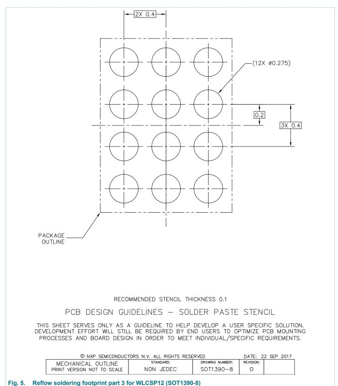
WLCSP12, wafer level chip scale package; 12 bumps; 0.4 mm pitch; 1.65 mm x 1.25 mm x 0.525 mm body (backside coating included)
