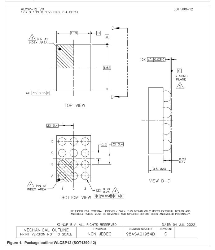
WLCSP12, wafer level chip-size package, 12 terminals, 0.4 mm pitch, 1.62 mm x 1.19 mm x 0.56 mm
