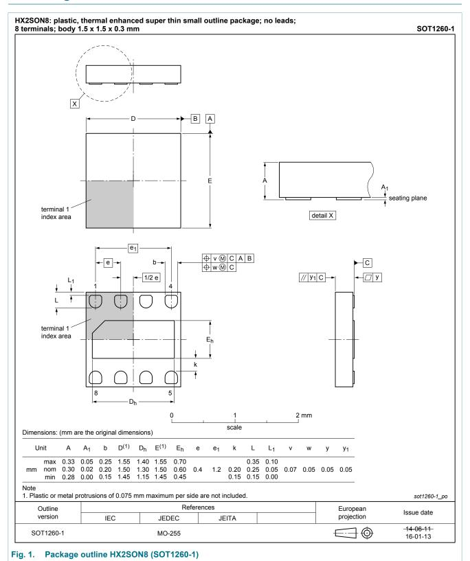
plastic, thermal enhanced super thin small outline package; no leads; 8 terminals; body 1.5 mm x 1.5 mm x 0.3 mm
