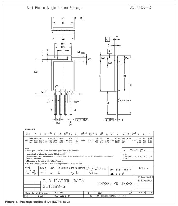
SIL4, plastic single in-line package, 4 terminals, 1.8 mm pitch, 11 mm x 7.4 mm x 1.95 mm body
