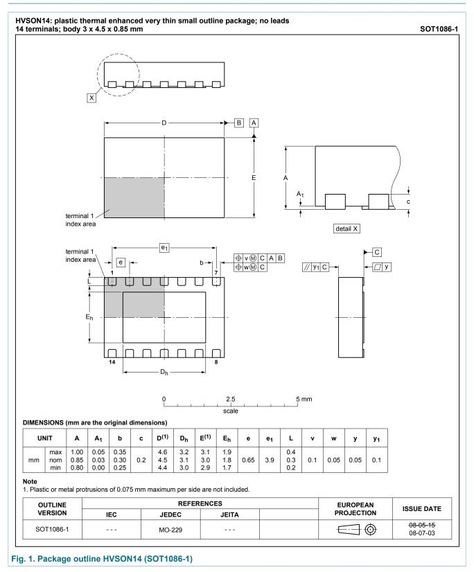
plastic thermal enhanced very thin small outline package; no leads; 14 terminals; body 3 x 4.5 x 0.85 mm
