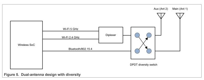
The dual-antenna design can also include an auxiliary Wi-Fi antenna that supports diversity, and a separate antenna for Bluetooth/802.15.4 radio without antenna diversity. In this configuration, the Wi-Fi and Bluetooth/802.15.4 radios can operate simultaneously given the appropriate antenna isolation.
