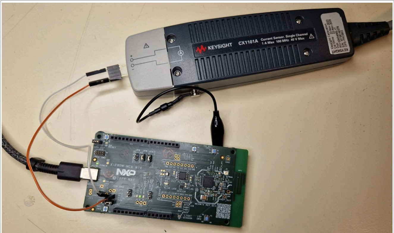
Figure 15. FRDM-MCX W71 board, current probe connected to JP2:1-2 example
