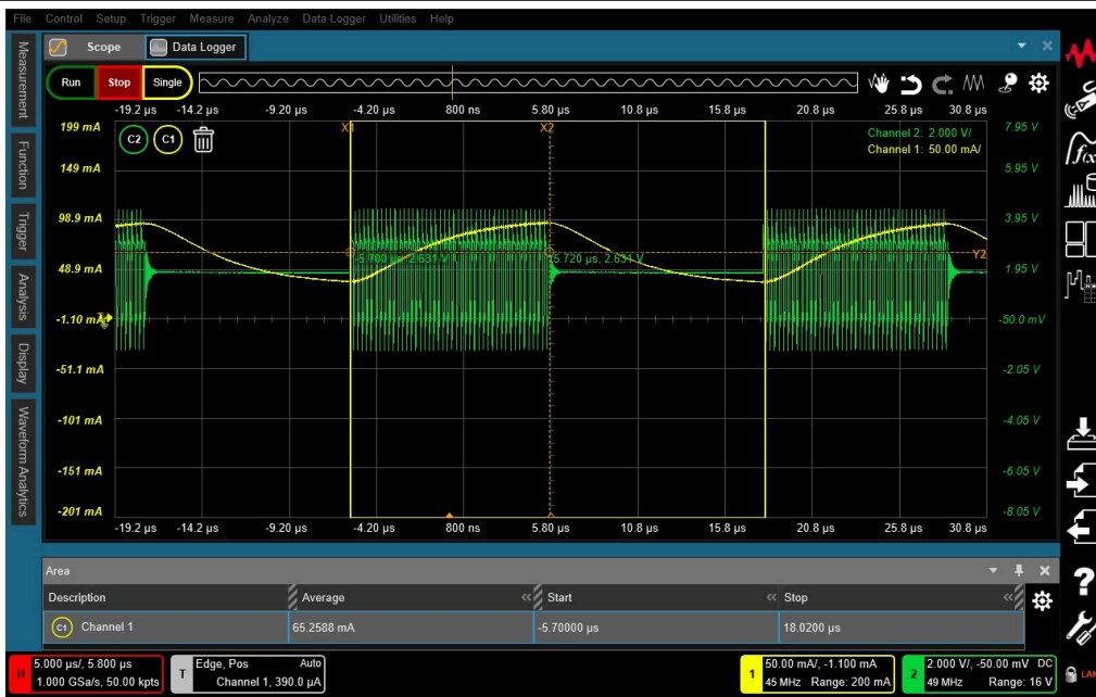
Figure 26. DC-DC Normal Drive Strength
