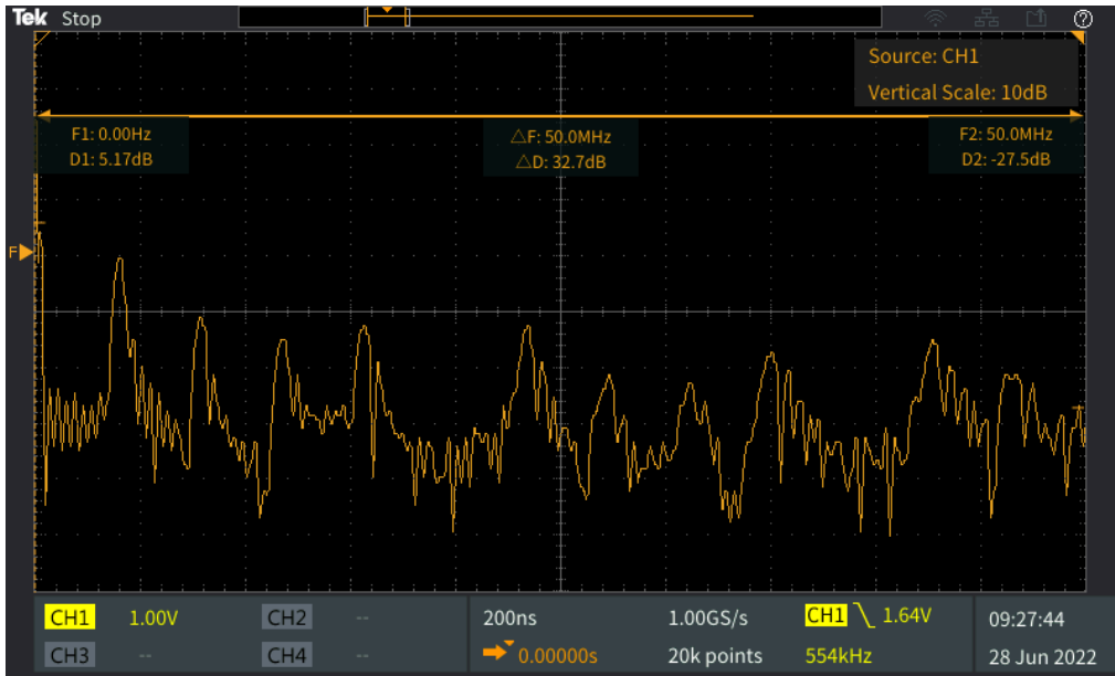
Figure 22. DC-DC frequency stabilization off, DCDC_OUT = 1.8 V
