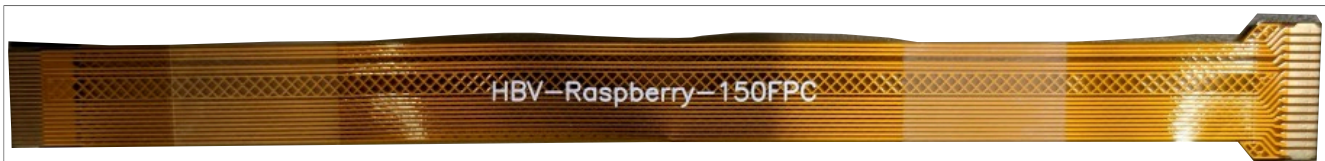
Figure 5. 22 pin (0.5 mm pitch) to 15 pin (1 mm pitch) FPC cable
