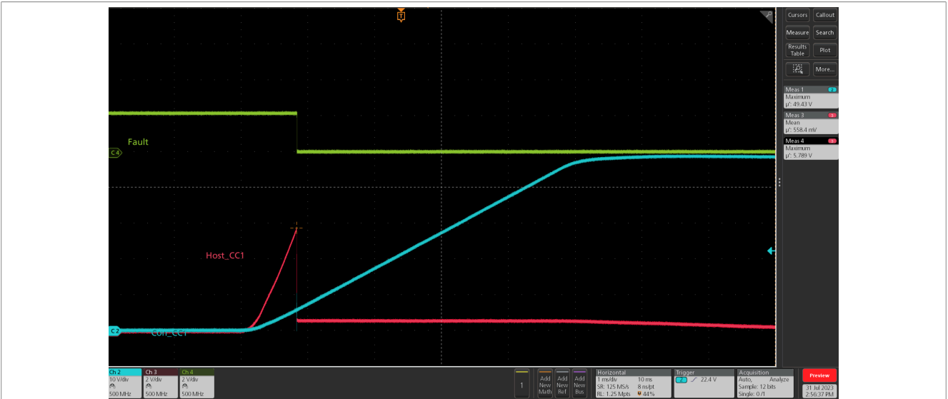
Figure 5. NX48P0407 CON_CC OVP test
