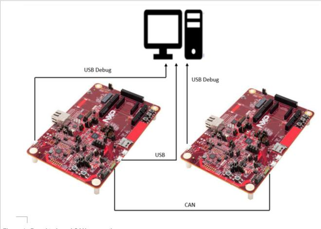
Figure 4. Board to board CAN connections
