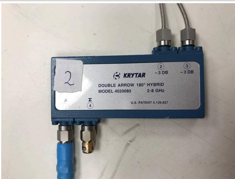
Figure 19. Example of the Balun used for the different measurements
