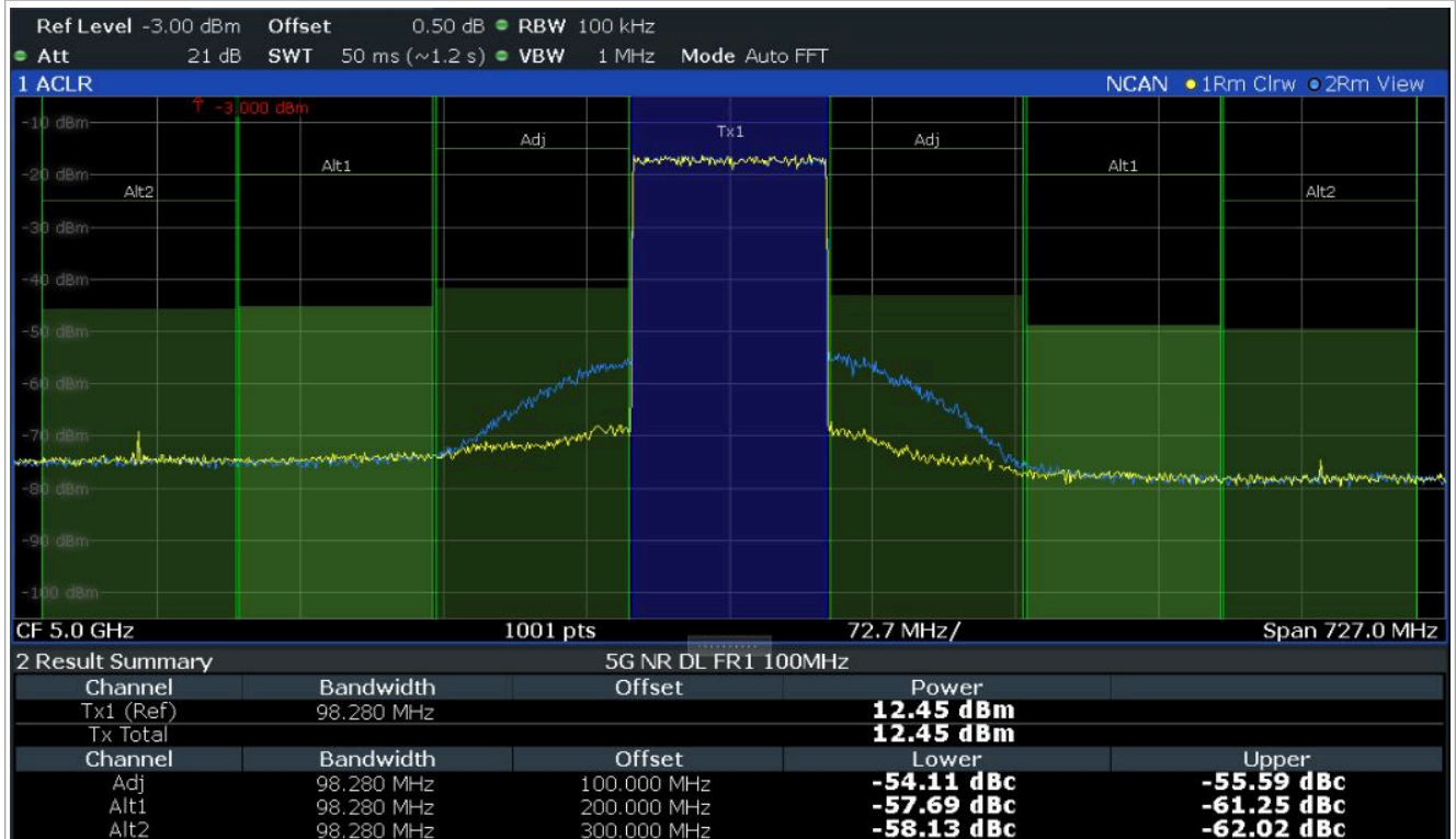
Figure 19. BTS6403C ACLR DPD vs none-DPD at 5.0 GHz center frequency and P out 12.5 dBm, CF 10 dB.
