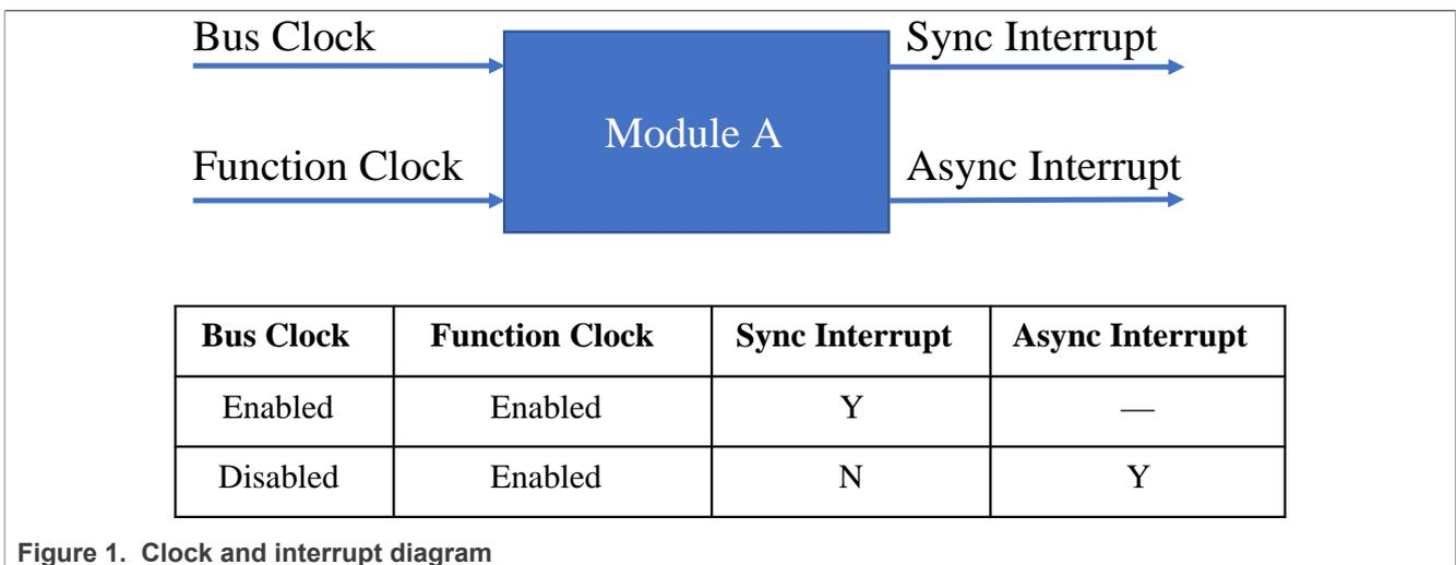
Figure 1 shows a clock and interrupt diagram. For some low-power-mode cases, the bus clock is shut down. To wake up the whole system from those low-power mode cases, the asynchronous interrupt can be used. Meanwhile, make sure that the power supply of this module is turned on during the low-power mode.
