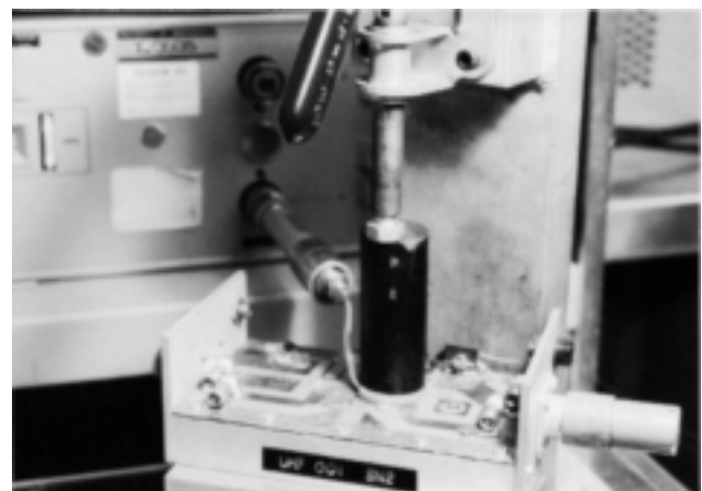
Figure 12. Adapter Used To Measure Circuit Impedance From Package
