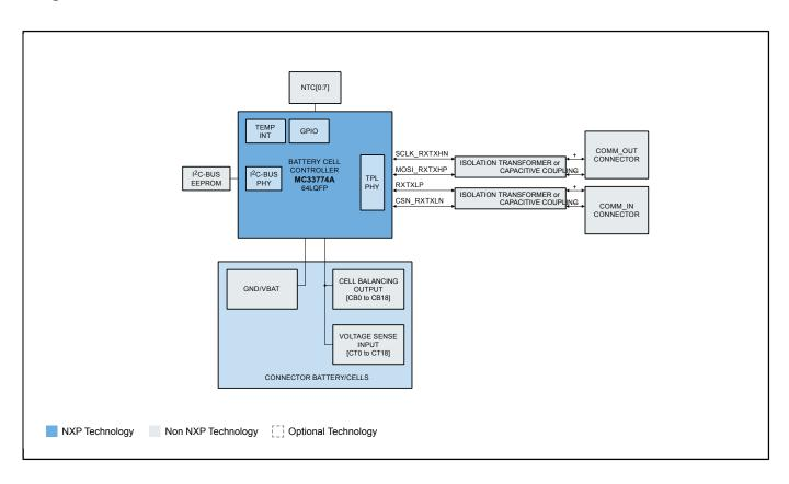
View additional information for MC33774ATA Evaluation Board with Isolated Daisy Chain Communication.
