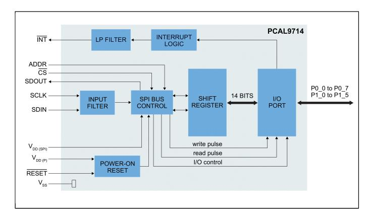
View additional information for 14-Bit SPI I/O Expander with Agile I/O Features.
