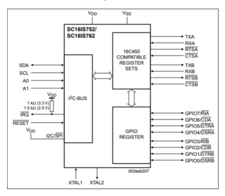
SPI Interface SC16IS752/762 Block Diagram
