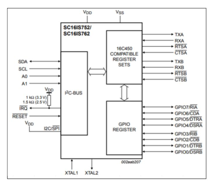
SPI Interface SC16IS752/762 Block Diagram
