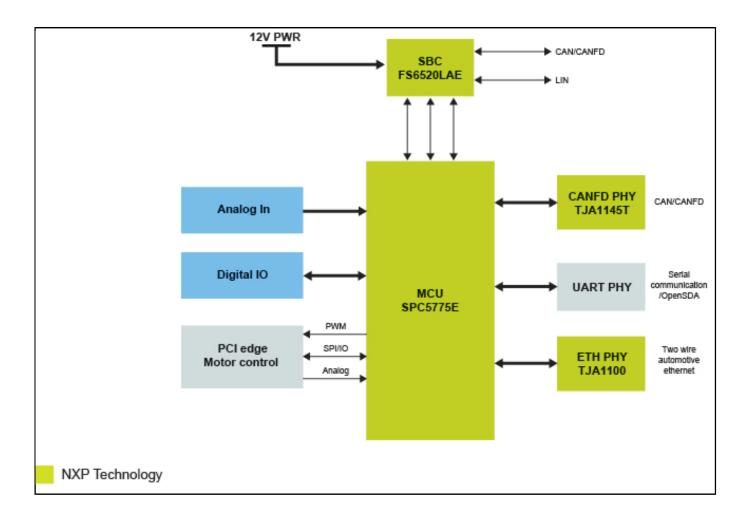
View additional information for MPC5775B/E low-cost BMS and Inverter Development Board.
