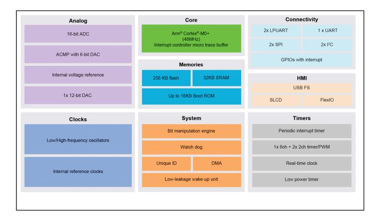
View additional information for MCX C14x/24x/44x MCUs with Arm® Cortex® M0+, Entry level MCUs with USB, Segment LCD and Classical Peripherals.
